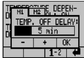
If both the sun- and the temperature-dependent controls are activated, the temperature function will only issue an Up command when the temperature is too low. Other sunshade functions are controlled by the sun function.
