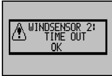
Wind sensor 2 has not sent any signals for 48 hours. Rotate the vane anemometer to check the sensor.
