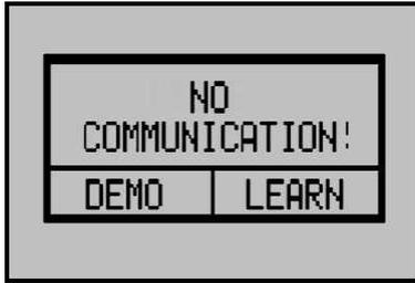
Now, you can select between demo and teach-in mode. In the demo mode, no radio connection between the operator and display element and control unit can be established. Therefore, control operations or configuration steps cannot be performed. If the operator and display element has not been “taught-in” with the connection box, select the teach-in mode by pressing the ‘TEACH-IN’-button.
