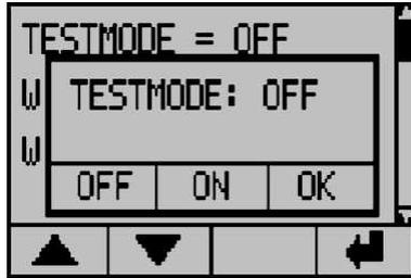
Continuous operation of the control in the test mode is not permissible.
