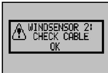
Wind sensor 2 cannot be detected. Check the wiring. As long as the wind sensor is not detected, the Up command remains activated.
