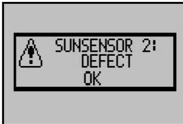
Sun sensor 2 is defective, not connected or short-circuited.
