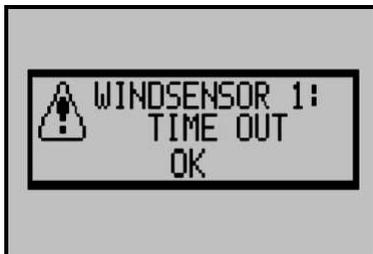
Wind sensor 1 has not sent any signals for 48 hours. Rotate the vane anemometer to check the sensor.
