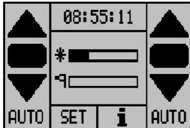
The status indication in the display center shows the currently measured sensor values. Touching this area will indicate details and other measured values.
