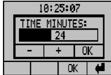
In this menu, you can change all user settings, such as wind, temperature, time, rain, run time and reverse time. Functions with only one setting can be directly changed. Other settings must be changed in a submenu. All settings are changed in a pop-up menu. With the arrows, you can access data currently not displayed on the screen.
