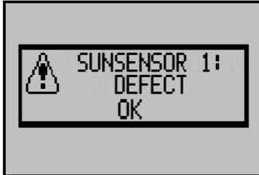
Sun sensor 1 is defective, not connected or short-circuited.
