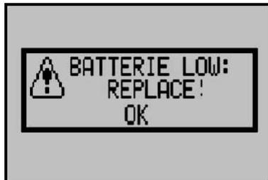
The batteries are almost completely discharged. Replace the batteries and only use batteries of the same type. If the battery charging capacity drops below 10 %, the operator and display element shows maximum contrast in order to ensure optimum readability. If you have purchased a unit with two-wire interface, the position of the slide switch on connection box and operator unit must be verified (see chapter, "Start-up / First steps").
