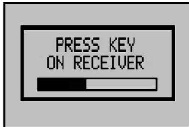
Make sure, the supply voltage for the connection box is turned on. If it is not, turn on the operating voltage and wait for at least 5 seconds. Then tap the ‘TEACH-IN’-button of the connection box (see wiring diagram) with an **insulated** screwdriver. The red LED next to the button will flash. If the operator and display element recognizes the connection box, the LED will stop flashing and the touch-screen will display the standard user interface. The system is now ready-to-operate.
