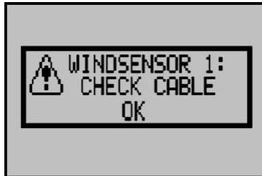
Wind sensor 1 cannot be detected. Check the wiring. As long as the wind sensor is not detected, the Up command remains activated.
